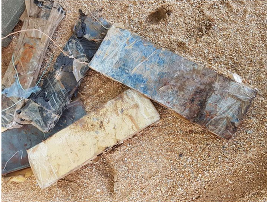
Picture 1: examples of pressure plates recovered in Gwoza area (September 2018)
