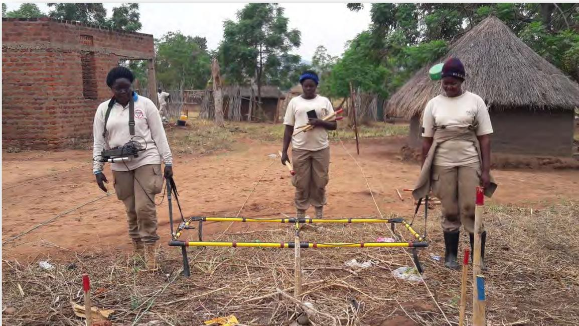
*The clearance of cluster munitions is done using “large loop” detectors which can be calibrated to discriminate the size of signals and thereby allow for swift clearance as only the targets that generate a reading less than that of a cluster munition can be ignored.*
