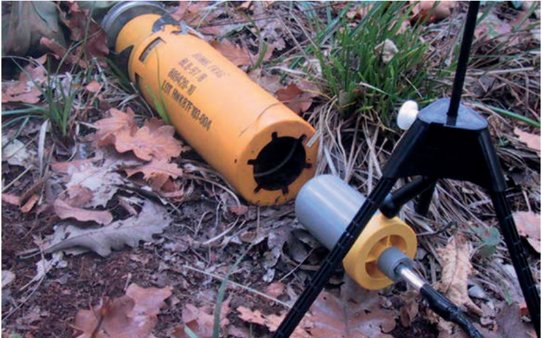
Safe Disposal of UXOs: Thanks to the Swiss developed SM EOD-Systems UXOs can be destroyed contact-free (c) DDPS
